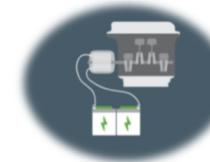
All four electric vehicle types use regenerative braking to charge the battery. While braking, the motor is still spinning even though the car is trying to slow down.
