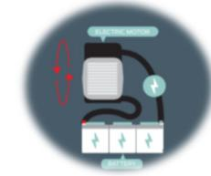
Regenerative braking captures this typically wasted energy to create electricity, which charges the battery.
